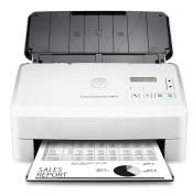
Scan resolution: Up to 600 dpi (color and mono, Sheetfeed) Hardware; Up to 600 dpi (color and mono, Sheet-feed) Optical.
